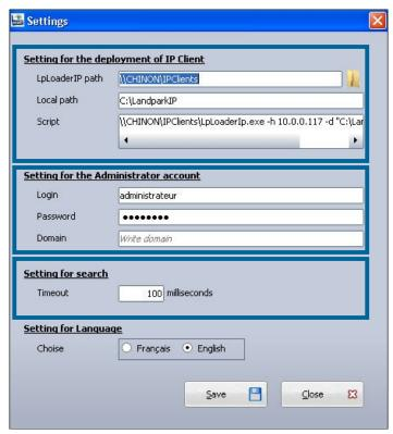
The application's settings panel lets you choose the folder where the deployment files are to be found, by using the « Browse » button. The deployment files are « LpServicelpClient.exe » and « ParamClient.ini ».
